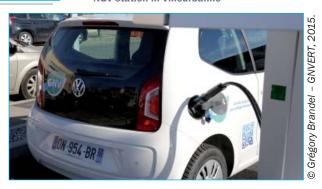
User constraints must be taken into account: thus, as regards to electric vehicles, terminals must allow for accelerated, slow or semi-accelerated charging in order to meet the needs of a whole range of possible uses of charging stations.
